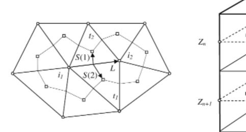
Velocities on cells (squares), scalars on vertices (circles) Medial-dual control volumes around vertices are hexagonal on equilateral meshes
