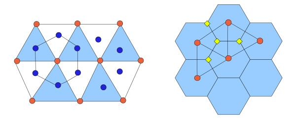
In reality, on uniform meshes  $(L_s \mathbf{u})_0 = (\mathbf{u}_1 + \mathbf{u}_2 + \mathbf{u}_3 - 3\mathbf{u}_0)/3$ , i. e., it is a filter operator. -- implement as filter (harmonic and biharmonic). But: it deviates from Laplacian on general meshes.
